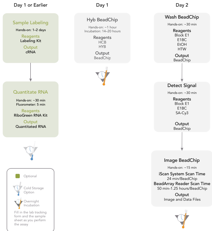
Figure 1 Direct Hybridization Assay Workflow
