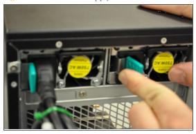
3 Push the new power supply into the slot and make sure that it is seated properly.
