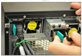
4 Attach the power cord to the power supply.
