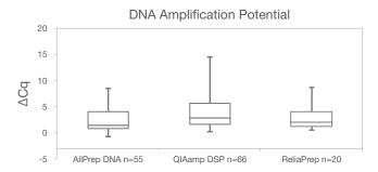
Figure 2: DNA Quality is Similar Across Extraction Kits—At least 20 samples were processed with each DNA extraction kit. DNA was qualified by qPCR. The  $\Delta$ Cq value indicates the difference in Ct value between each sample and that of a non-FFPE reference gDNA.
