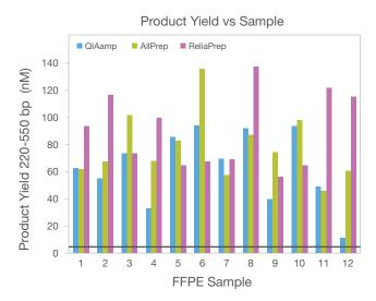
Figure 3: Product Yield After Library Prep—Following PCR purification, libraries within the 220–550 bp range were quantitated on a Fragment Analyzer. The black line indicates the threshold (4 nM) for a passing sample.
