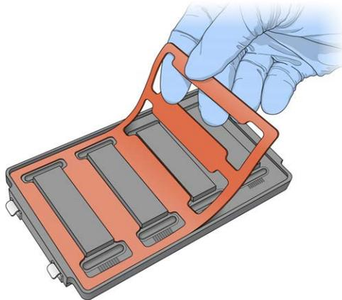
— Make sure that the Hyb Chamber gaskets are properly seated.
