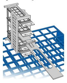
To ensure uniform coating, place the staining rack on the center of the tube rack. Avoid the raised edges.
