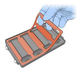
2 Dispense 400 µl PB2 into each of the eight humidifying buffer reservoirs in the Hyb Chamber.
