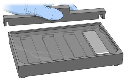
9 Place a clean LCG glass back plate on top of the clear spacer that is covering each BeadChip. Make sure the beveled edge of the LCG glass back plate is facing the barcode.
