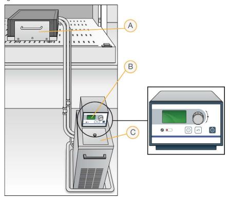
Figure 50 Water Circulator Connected to Chamber Rack
