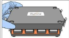
5 Close the Hyb Chamber clamps in this order: top-left, bottom-right, top-right, and then bottom-left. Make sure that the lid is secure and even on the base (no gaps).
