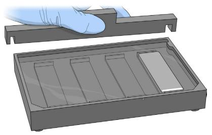
Place a clean LCG glass back plate on top of the clear spacer that is covering each BeadChip. Make sure the beveled edge of the LCG glass back plate is facing the barcode.
