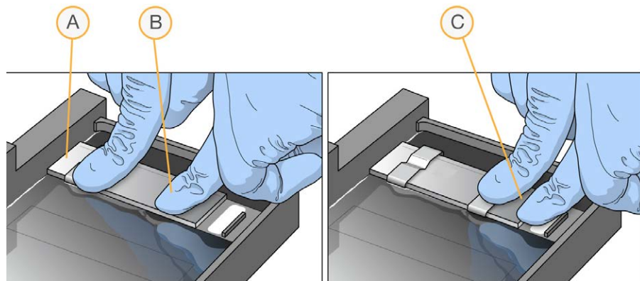
Figure 30 Securing the Metal Clamps
