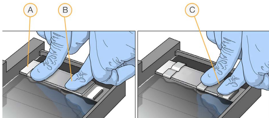
Figure 70 Securing the Metal Clamps
