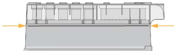
Figure 1 Maximum Water Line
