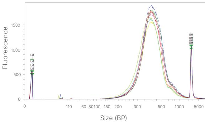
Figure 2: Insert size distribution of eight libraries prepared with automated workflow—Overlay of eight traces from the LabChip GX Touch Nucleic Acid Analyzer representing eight different libraries prepared with the automated Illumina DNA Prep workflow. The libraries represent two DNA isolation replicates from the adult, donor 1, sample and two DNA isolation replicates from the child, donor 3, sample. Two replicates were generated from each DNA isolate producing a total of eight libraries.
